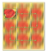
100% Linear scan Automatic recording of the total print format at constant camera travel. Zoom setting can be changed during scan mode. Adjustable scan speed.
