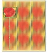
Slow motion scan Automatic continuous scanning (slow-motion) in web direction. Camera can be positioned during scan mode across the printing web. With the new BACK-function Kara return of the scan direction is possible Adjustable slow motion speed
